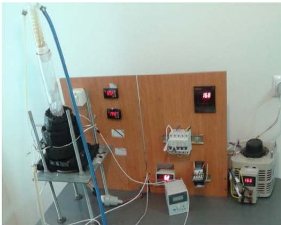
Fig. 8 The real image of boiling set up
