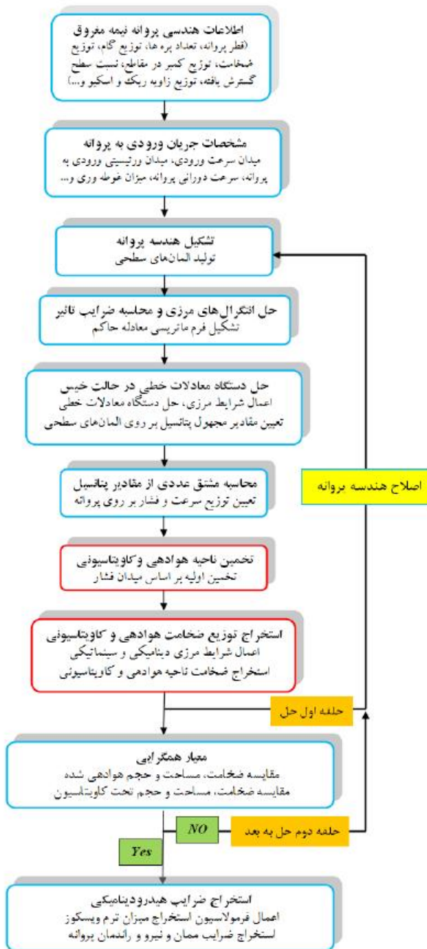
Fig. 7. The flowchart of ventilation-cavitation flow around surface piercing propeller
