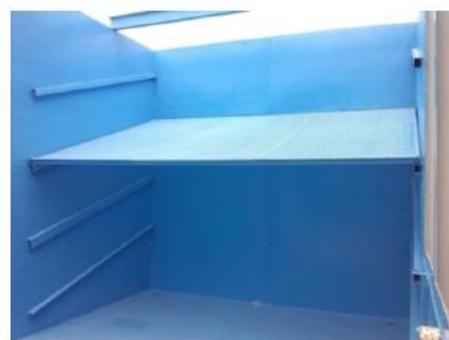
Fig. 5. The damper system of wave tank
