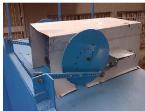
Fig. 4. Motor and moving mechanism of the paddle
