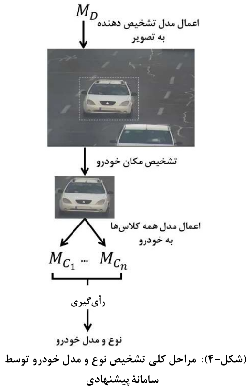
(Figure-4): The flowchart of proposed system for vehicle make and model recognition
