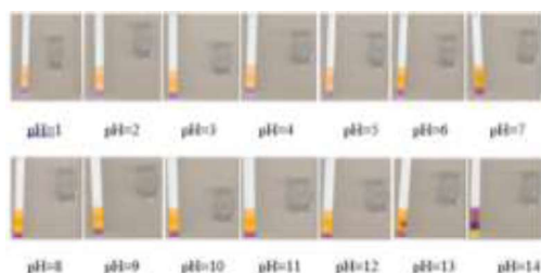
Fig. 4. Schematic of the solutions in cells and pH paper in different steps of titration, for indicator Phenol phtalein.
