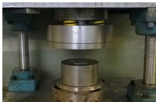
Figure 2. The fabricated die with the metal die.
