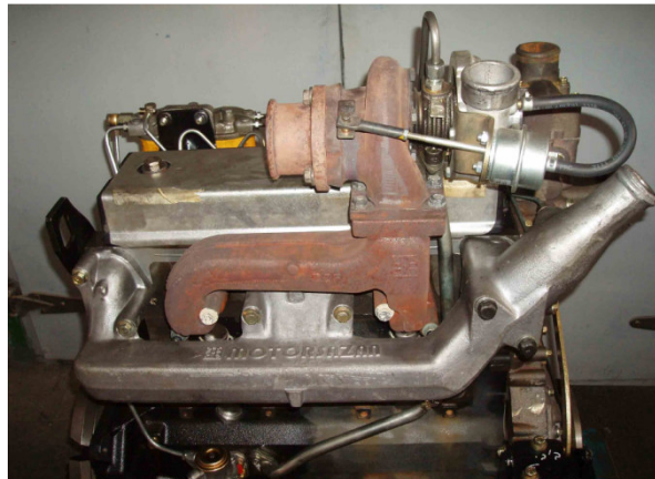
Figure 1- MTI4.244 diesel engine produced by Tabriz Motorsazan Company
