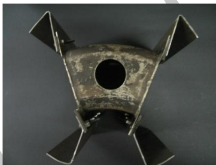
Figure 10- Combustor sector and test section holders
