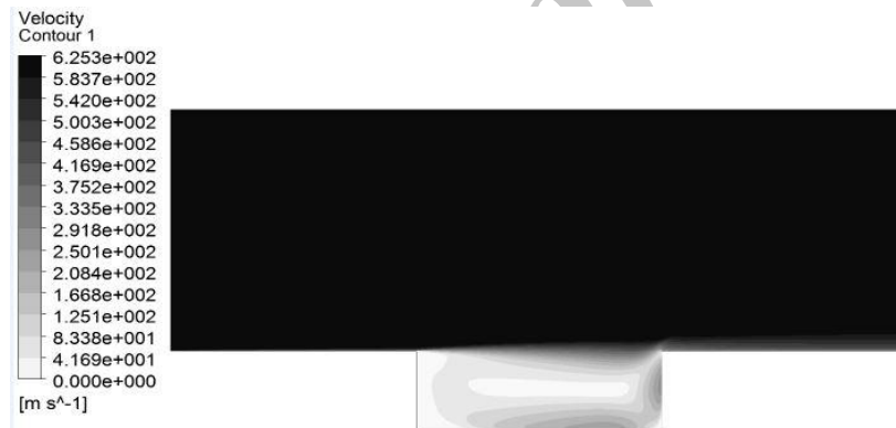
Figure 13- Non-dimensional velocity contour for Mach 3
