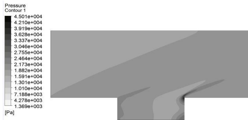
Figure 12- Static pressure contour for Mach 3
