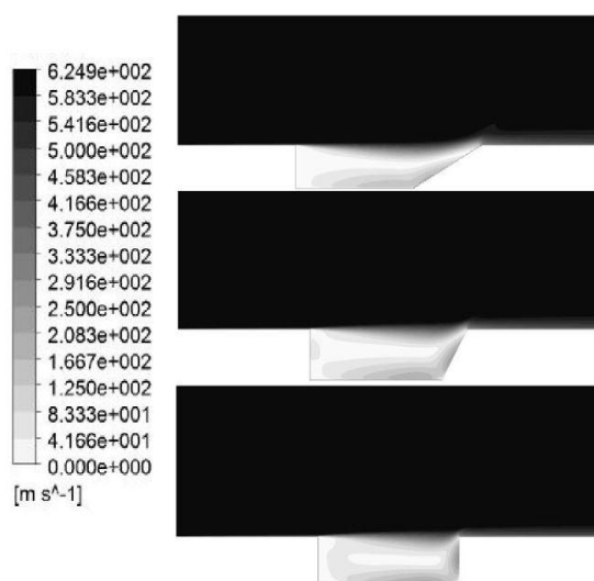
Figure 15- Comparison of speed contour for three angles (respectively from above) 30, 60 and 90 degrees
