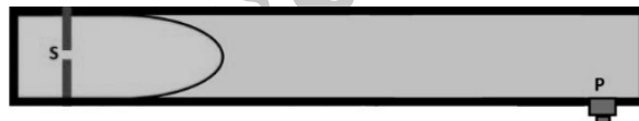
Figure 2- Schematic diagram of the closed channel (combustion chamber). Points S and P indicate the location of spark plug and pressure sensor, respectively
