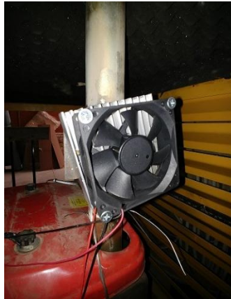
Figure 3- Exhaust thermoelectric waste heat recovery system
