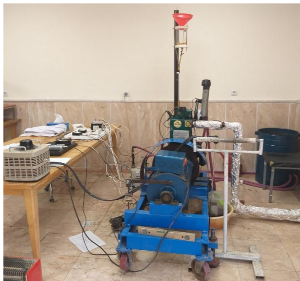
Figure 1- Diesel engine used to test emission and performance
