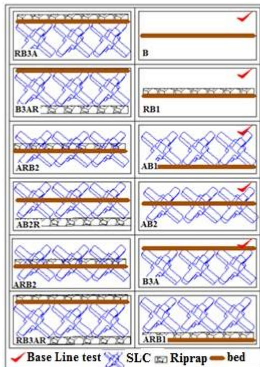
Fig. 5- Different arrangement for riprap & SLC
