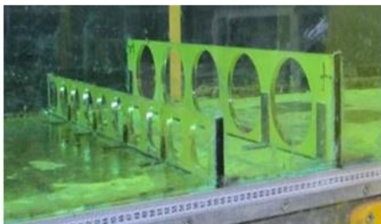
Fig.4- View of perforated sills. A) Schematic of perforated sills. B) View of the plexiglass perforated sills in the experiments
