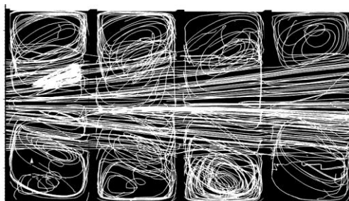
Fig. 19- The top view of flow pattern in the Daniel fishway with a baffle angle of 60 °
