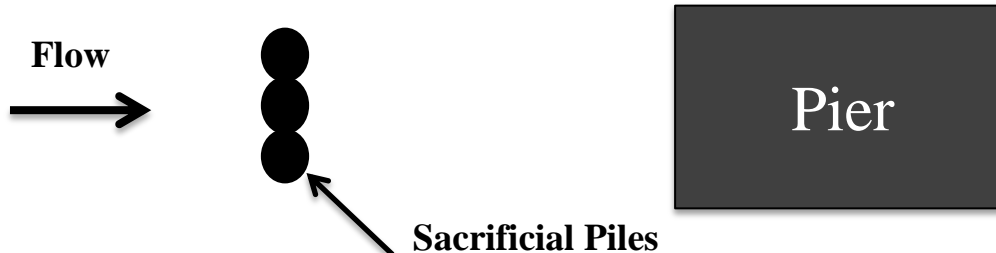
Fig. 1- Sketch showing arrangement of sacrificial piles in front of pier, from Haque et al. (2007)
