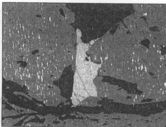
Fig. 5 Photomicrograph shows gold (electrum) grain within chalcopyrite.
