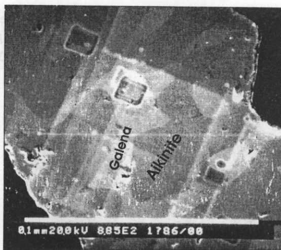
Fig. 7 Back-scattered electron photograph of intergrowths or exsolution of aikinite and galena (sample 3-70, Au).
