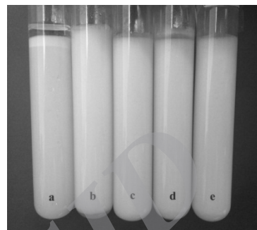
Fig 4 Photos of emulsion containing (a) 0%, (b) 0.25%, (c) 0.5%, (d) 0.75% and (e) 1% gum after 28 days at 4.
