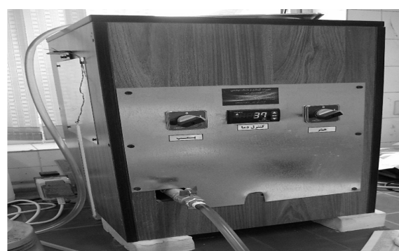
Fig D Water bath circulation
