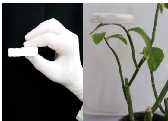
Fig 5 Production of cellulose nanofibers aerogel from date palm.
