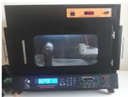
Fig 1 Electrospinning device used in this study
