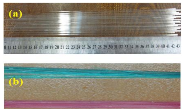
Fig. 1 The glass micro-tubes a) before and b) after the filling using healing materials
