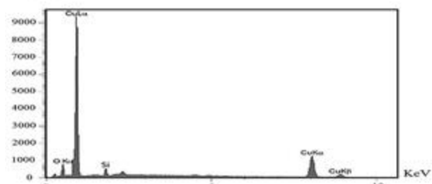
Fig. 7 SEM micrograph of the SZ (a), EDS composition analysis(b)
