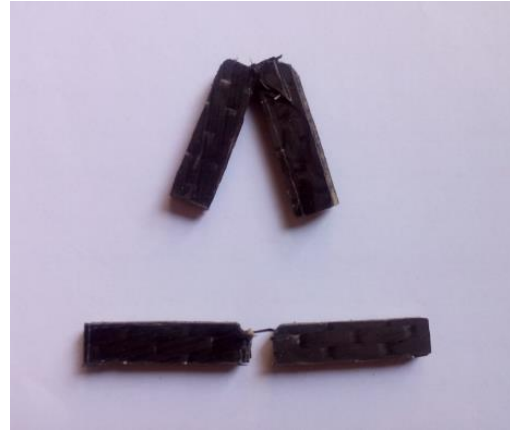
Fig. 4 Sandwich panel specimens without self-healing materials (tester) after CHARPY impact test
