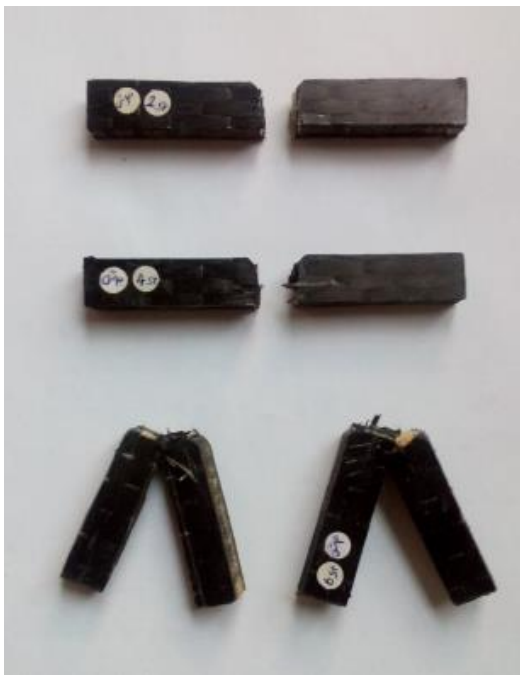
Fig. 11 Specimens after CHARPY impact test: 1 st row 2 pairs micro tube, 2 nd row 4 pairs micro tube, right of 3 rd row 6 pairs micro tube and left 3 rd row undamaged (control)
