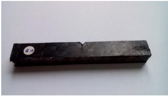
Fig. 3 Damaged specimen using for CHARPY impact test
