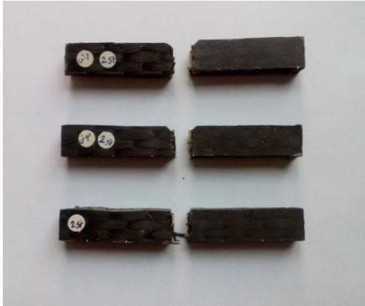
Fig. 5 Sandwich panel specimens with 2 pairs of self-healing micro tube after CHARPY impact test
