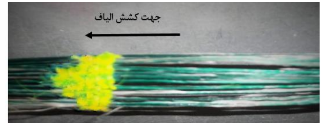
Fig. 11 Status of Colored Particle in Preimpregnated Fiber After Exiting from Mold
