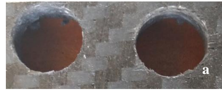
Fig. 1 Hole entry in CFRP (Diameter: 10 mm, Spindle Speed: 1400 rpm, Thickness: 3 mm) a) Feed rate: 0.28 mm/rev, b) Feed rate: 0.11 mm/rev
