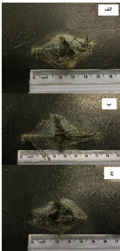
Fig. 6 Damaged area of composite with a) 0, b) 0.3 c) 0.5 wt.% silane modified GNPs.
