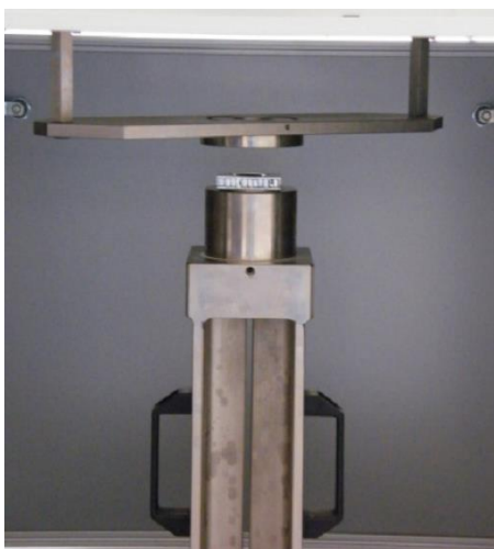
Fig. 5 Clamping system of specimen for impact test
