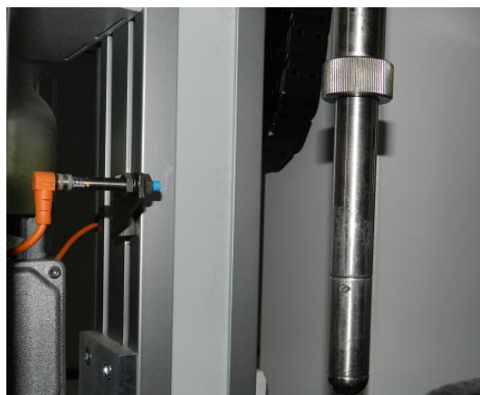
Fig. 4 Spherical Impactor with strain gauge
