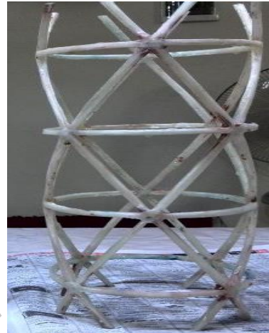
Fig.4 Lattice sample made using Teflon mold
