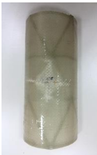
Fig. 14 Front view of lattice sample were tested
