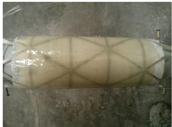
Fig. 9 Lay up of skin around ribs
