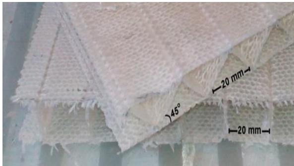
Fig. 4. The 3DIWKSCs with tow cross-sectional shape
