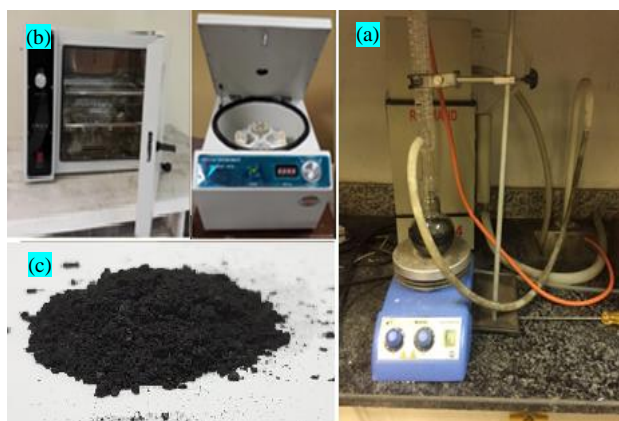
Fig. 1 Functionalization process of graphene, a) Reflux system, b) Centrifuge in right and oven in left of the image and c) Functionalized graphene powder.
