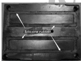
Fig. 1 Pressing die for constructing fiber metal laminates
