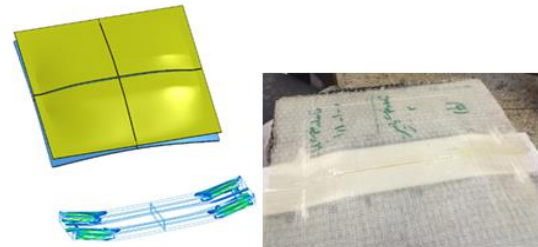
Fig. 20 Failure modes after performing bending test on the plates with connection type 2 (Numerical and experimental)
