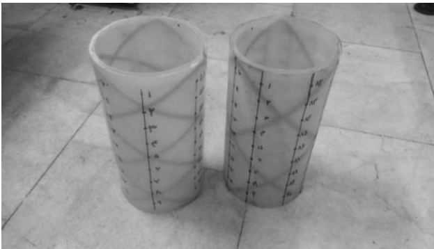
Fig. 6 Composite sandwich shell with lozenge core
