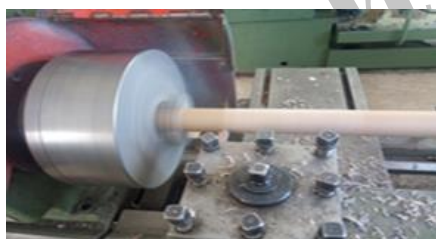
Fig. 2 machining of surface of mandrel for sizing
