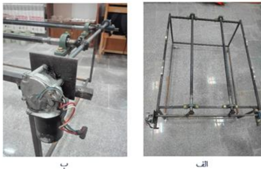
Fig. 3 A: tube rotor device B: Low speed 12Kw motor
