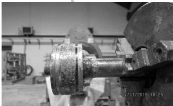
Fig. 9 Filament winding process of the nol rings
