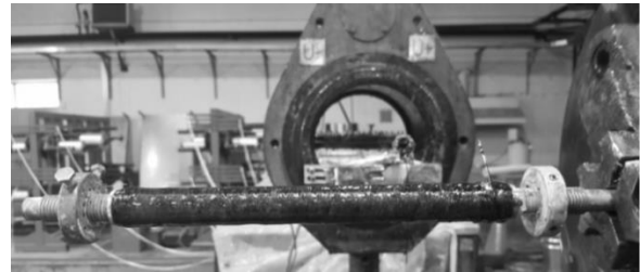
Fig. 4 Filament winding process of the cylindrical composite shell with embedded shape memory alloy wires
