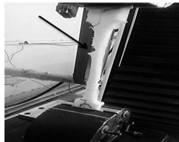
Fig. 9 Start of failure from sample surface during tensile test
