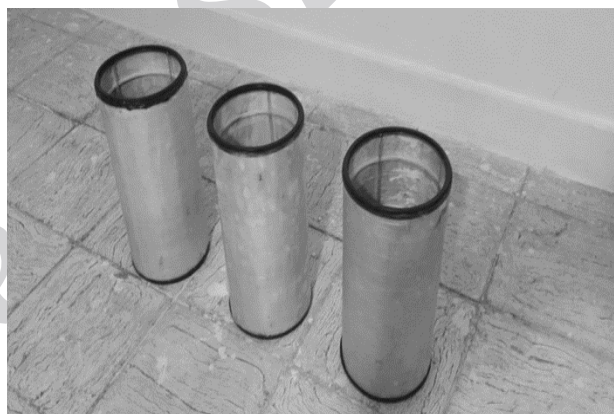
Fig. 2 Fabricated FML shells
