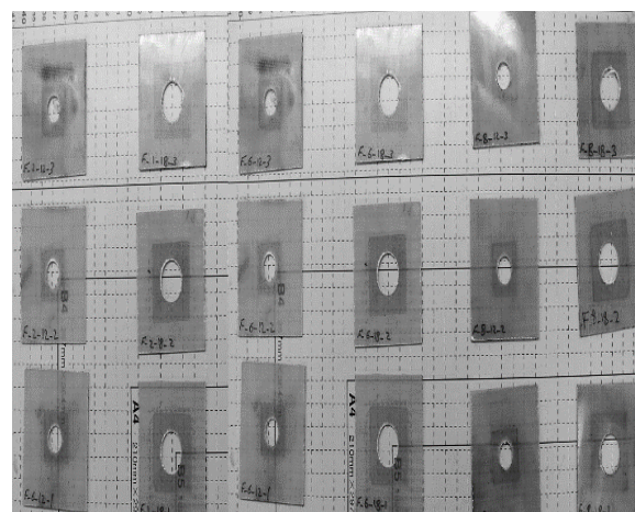
Fig. 7 Composite plate having circular hole with planer stiffener
