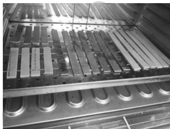
Fig. 3 Post-cure process of the specimens
