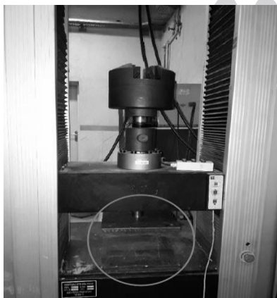
Fig. 5 Image universal testing machine for conducting a pressure test between two parallel rigid plates
