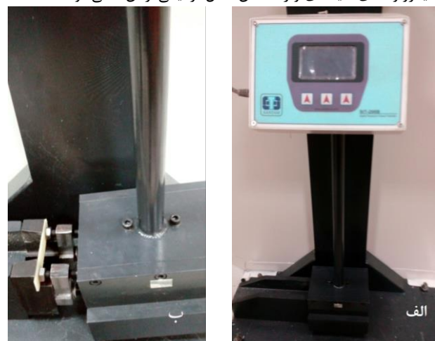
Fig. 2 a) Schematics of charpy impact test device and causing damage procedure.
