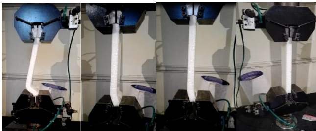
Fig. 21 Edgewise compression set – up and failure sequences of radome sandwich panel
