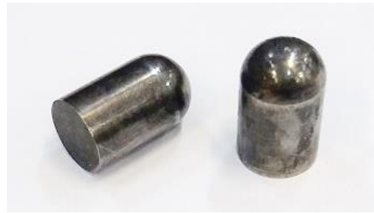
Fig. 2 Hemispherical projectile used in experiments
