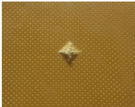
Fig. 9 Damage of the composite under impact velocity of 75 m/s
