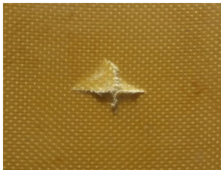
Fig. 10 Damage of the composite under impact velocity of 117 m/s
