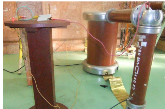
Fig. 3 High voltage test setup for measuring breakdown voltage and leakage currents.
