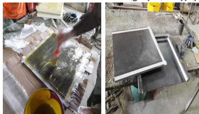
Fig.1 Fabrication of sandwich panels with different fiber Lay-ups
