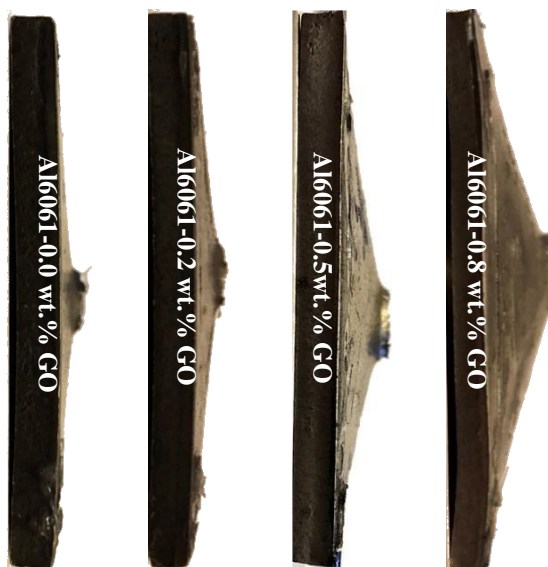
Fig. 11 Global deformation of aluminum alloy samples from the side view of the impact test
