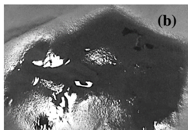
Fig. 2 preparation steps of graphene oxide powder: a) sonication of GO in acetone with ultrasonic probe and b) mixture sprayed on aluminum foil
