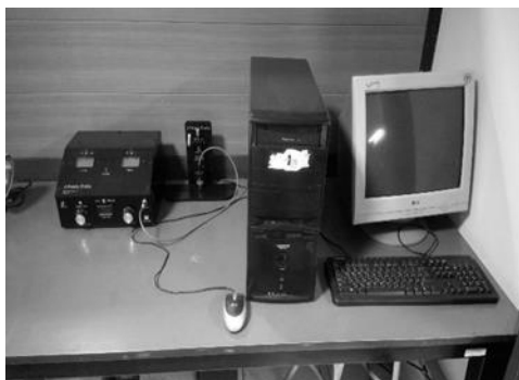
Fig. 3 Four Probe Point Electrical Conductivity Test Device
