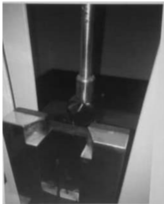
Fig. 2 Charpie's Impact Test Device
