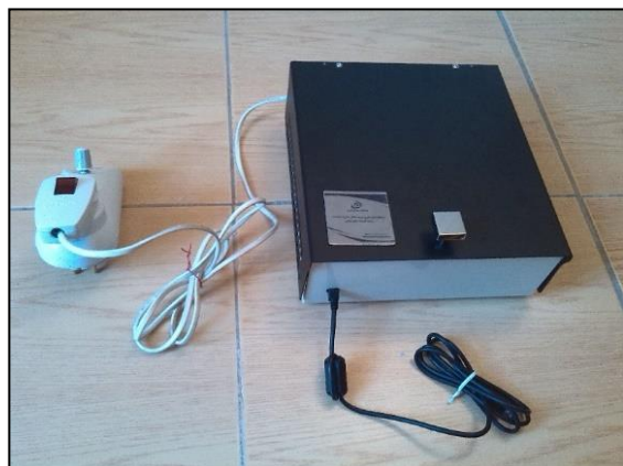
Fig. 12 Heat transfer conductivity measuring device used in experiments
