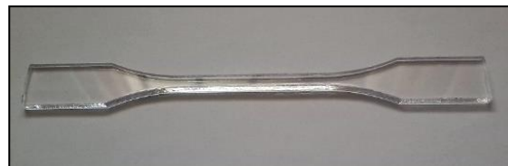
Fig. 9 PMMA sample for tensile test.
