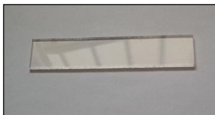
Fig. 8 PMMA samples for contact angle test.
