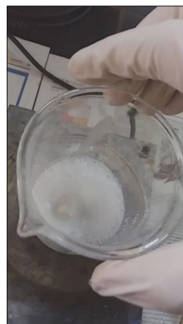
Fig. 6 Dissolving polymer in propanone (acetone).
