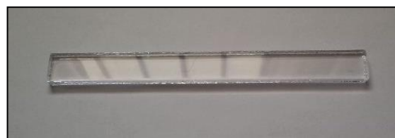
Fig. 11 PMMA samples for flexure test ( 125 \times 12.7 \times 3.2 \text{ mm}^3 )
