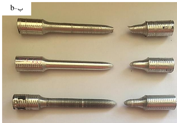
Fig.8 A number of broken samples in the a) Compression test b) Tensile test.
